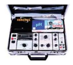
Based on advance electronic technology for water analysis, pollution control, laboratory analysis, soil testing etc. Complete unit is housed in a briefcase to work on battery rechargeable cum mains. Unit is supplied without O.R.P. electode with instruction manual.
