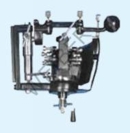
Weiber freezing microtome is used for cutting thin to semi-thin sections of fresh, frozen tissue and semi-thin sections from industrial products such as some textiles, paper, leather, soft plastics, rubber, powders, pastes and food products. The microtome is equipped with a stage upon which tissue can be quickly frozen using either liquid carbon dioxide, from a cylinder, or a low temperature re-circulating coolant. Some cooling systems also allow the knife to be cooled at the same time.
